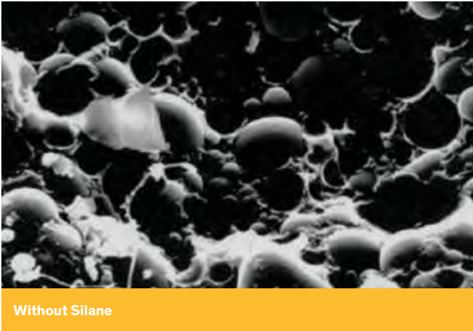
Figure 2: SEM image of silica-filled epoxy resin
