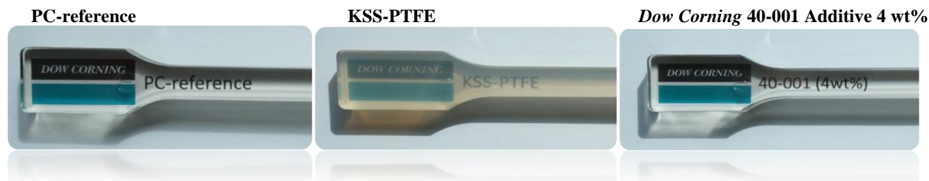
Figure 1: Demonstration of no influence of Dow Corning 40-001 Additive on polycarbonate optical properties, compared to KSS+PTFE formulation which showed strong haziness, typical for such formulations.
