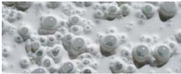
Glass beads in paint for road markings
